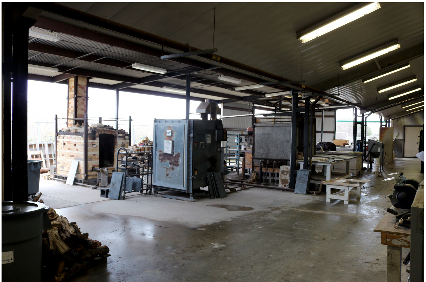
The 2298 square foot outdoor covered kiln yard with a Bailey Gas Kiln (center), a reduction cooling kiln (right), and a soda/salt kiln (left). The yard also contains a wood fire kiln, two Skutt barrel kilns, and a Bailey Raku Kiln.
